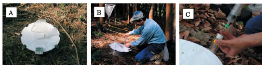
Figure T02-2 Measurement of greenhouse gas by flux method 4)
