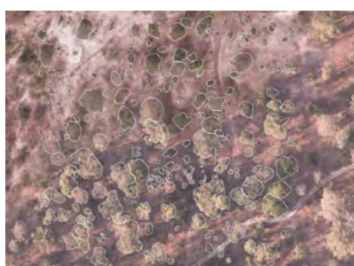
Figure T17-2 Extraction of crown polygon by stereoscopy of digital aerial photograph (dry dipterocarp forest in Kampong Thom, Cambodia)
